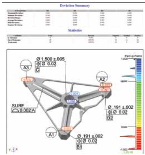
Verisurf X uses the CAD model as the nominal definition to generate custom reports in industry standard formats, including GD&T constraints and color deviation maps. A Database Write feature in the program formats and sends inspection information to SPC applications and PLM databases used by major manufacturers. The feature also supports Microsoft Access and SQL Server database formats for combining Verisurf inspection data with numerous enterprise databases.
