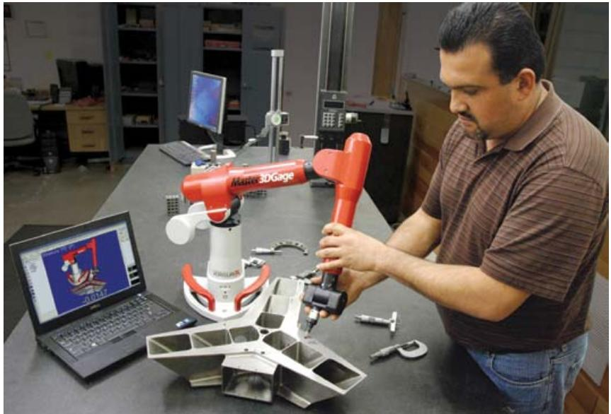
When problems occur, turn the arm into an investigation tool. Rather than inspecting parts or processes to a predefined plan, use it to query the part to determine where the problem lies and what its root cause is. The arm offers the flexibility to conduct “what-if” diagnosis to understand the cause and effect. *Source: Verisurf*
